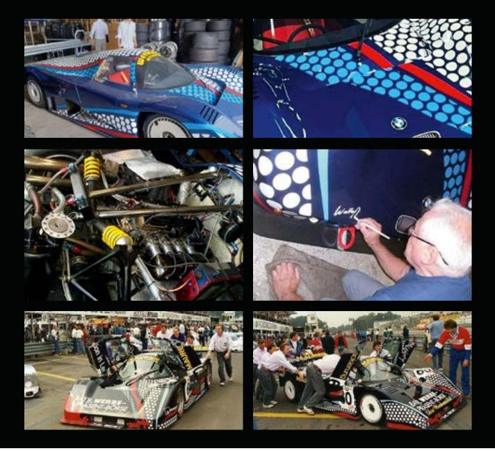
Developed under the supervision of Paul Rosche, the turbocharged BMW M12 four-cylinder engine displaced 2.0 litres and was capable of delivering 1,350bhp in qualifying trim with the boost at maximum. BMW had plenty of experience of using this type of engine in Formula 1, supplying the World Championship-winning Brabham team, though the Maurer C87's engine and transmission are unique to this car.
